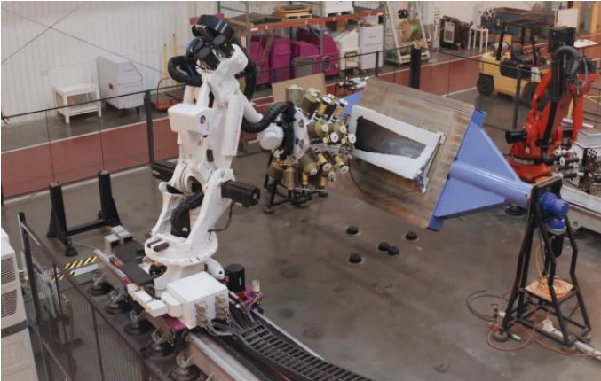
Composite Robotic Layup Machine 2015
